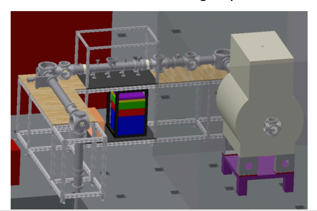
Penning trap uses electric and magnetic fields to trap short-lived charged particles
