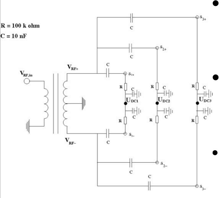
circuit diagram for connecting RF and DC voltages
