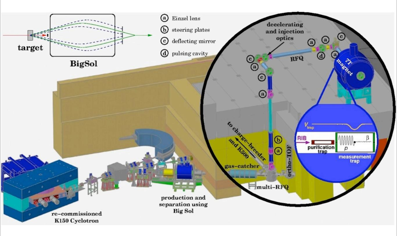
new beam line and Penning trap
